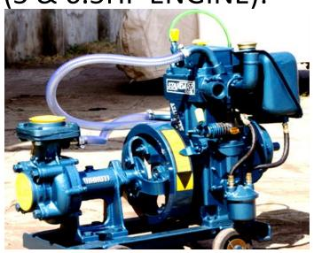
Mini Centrifugal Water Pump Oil Seal Type DB (china and mini water cooled engine):
